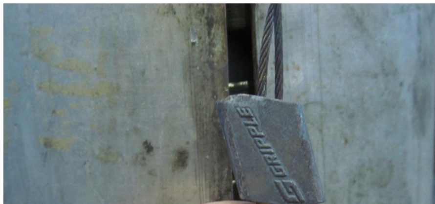
Figure 6 - Gripple S/S No. 2 unit after fire exposure for 60 minutes
