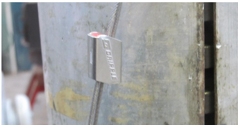
Figure 1 - Gripple (No. 2) cable connector, before fire exposure
