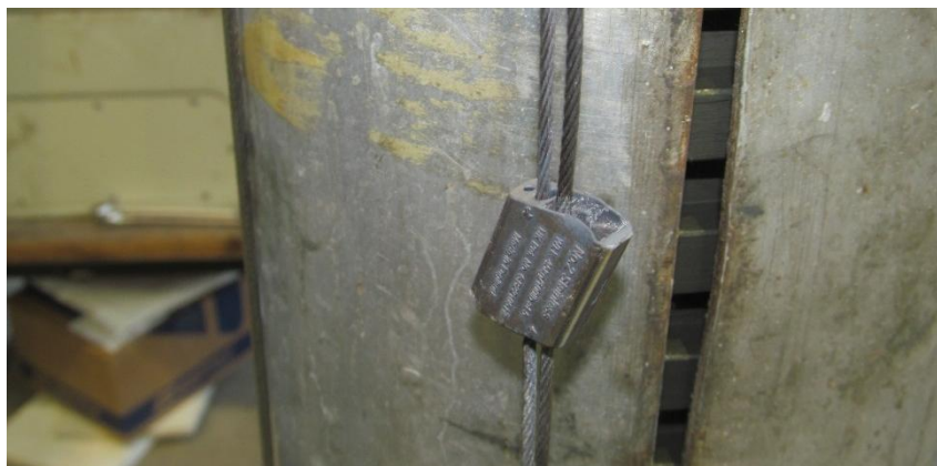
Figure 4 - Gripple S/S No. 2 unit after fire exposure for 30 minutes
